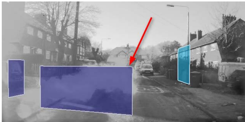
Figure 26: Cloud of smoke triggering Subcritical AEB Sequence 1 in January 2017. Still frame of the trigger time extracted from the stereo video recording with boxes indicating camera-detected objects. Red arrow highlights the object causing the trigger.
