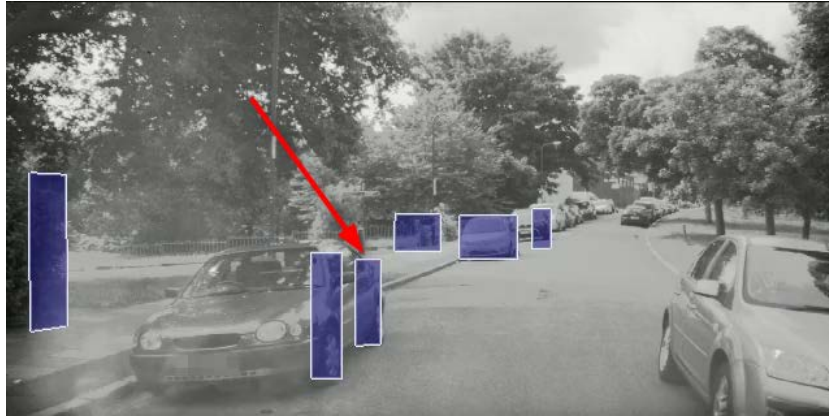
Figure 27: Corner of parked vehicle triggering Subcritical AEB Sequence 6 in July 2017. Still frame of the trigger time extracted from the stereo video recording with boxes indicating camera-detected objects.
