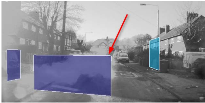
Figure 2: Cloud of smoke triggering Subcritical AEB Sequence 1 in January 2017. Still frame of the trigger time extracted from the stereo video recording with boxes indicating camera-detected objects. Red arrow highlights the object causing the trigger.
