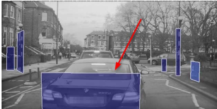
Figure 25: Leading vehicle triggering Subcritical AEB Sequence 3 in February 2017. Still frame of the trigger time extracted from the stereo video recording with boxes indicating camera-detected objects. Red arrow highlights the object causing the trigger.
