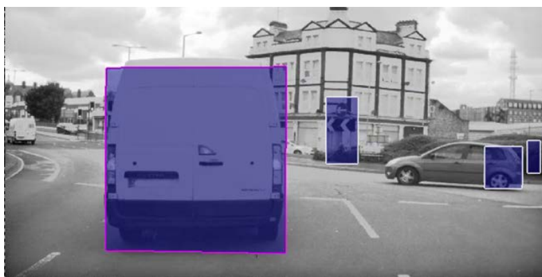
Figure 30: Driver brake application triggering DHB Sequence 5. Still frame of the trigger time extracted from the stereo video recording with boxes indicating camera-detected objects.
